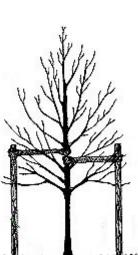
**Staking** the tree is not always necessary, but is recommended for roadside and urban planting. The ties should be tight enough so they do not rub the trunk and loose enough for the tree to flex in the wind. Staking is only for initially establishing the tree and should be removed after one year.
