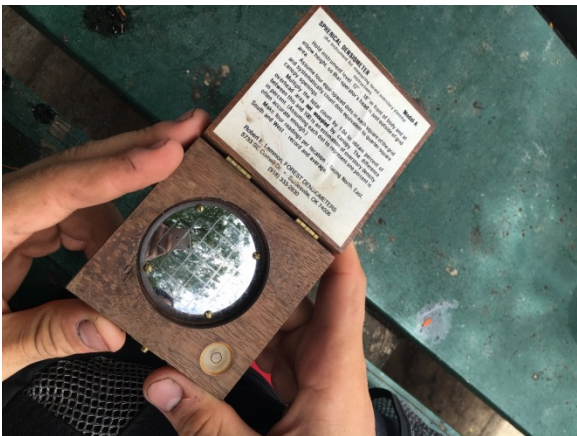
Figure 1. Spherical densitometer used to measure canopy coverage
