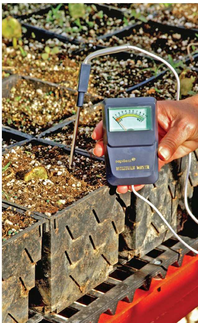
Figure 11.14 —Many types of tools can be used to help test and assess the effectiveness of water application, including this moisture meter. Visual and tactile assessments are more prevalent in tropical plant nurseries, however, and can be quite effective when carried out by trained staff. Photo by Thomas D. Landis.
