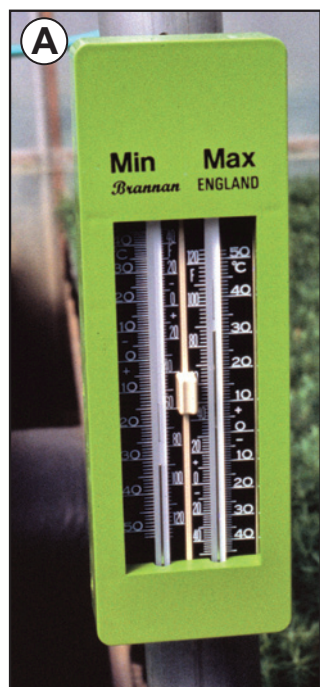
Figure 5.13 —Monitoring and controlling temperature is critical to successfully growing a crop of tropical plants (A). Many nurseries use small, programmable, self-contained temperature sensors that record daily maximum and minimum temperatures (B and C). Photo A by Thomas D. Landis, and photos B and C by David E. Steinfeld.
