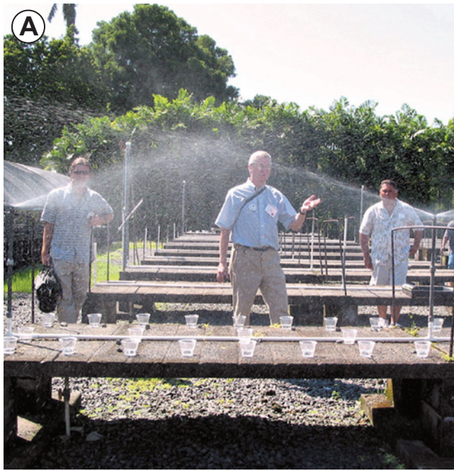
Figure 11.16 —Periodic checks of water distribution can easily be done with a “cup test” in which cups are arranged in a grid pattern (A). The depth of water in the cups is measured after a standard watering period (B). Photo A by Kim M. Wilkinson, and photo B by Thomas D. Landis.
